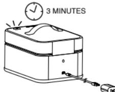
5. Take out items when the process completes with indicator stop flickering. Tray can be kept inside for next use.
